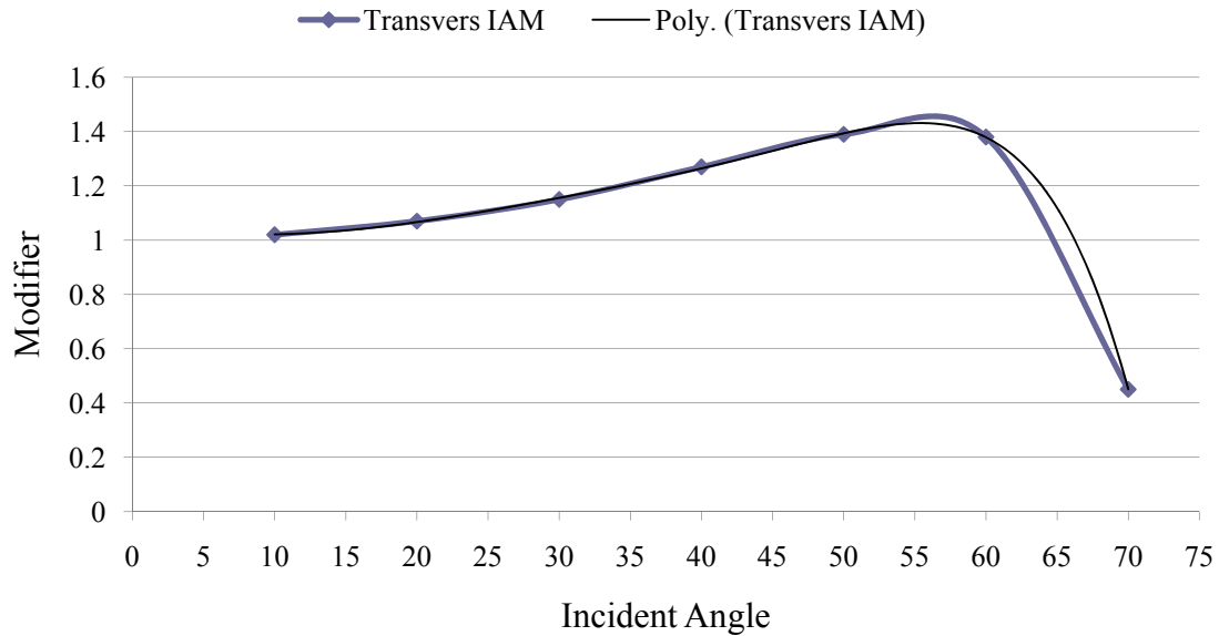
Figure 2.13 Transverse incident angle modifier for different solar incident angles from the SRCC data
